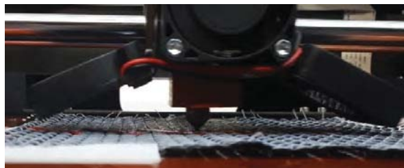
Figure 1. 3D printing of PCL interlayer material on the reinforcement fabric using FFF method
