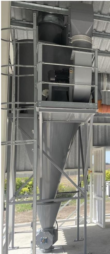
Fig 4. The produced dust separator cyclone
