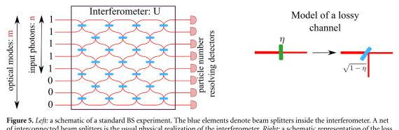
of interconnected beam splitters is the usual physical realization of the interferometer. *Right:* a schematic representation of the loss model we use in this work. On the left side of the diagrammatic equation, we see a lossy channel on a single mode, with particle transmission probability  $\eta$ . On the right side of the equation, one can see the applied beam splitter that mimics such a channel. The transmitted beam labeled by  $\sqrt{1-\eta}$  is not measured.
