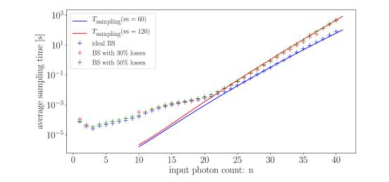
**Figure 6.** Performance of the developed BS simulation design executed on two *AMD EPYC 7542 32-Core Processor* servers, each server containing of 2 CPU nodes and two Xilinx Alveo U250 FPGA cards. The averaged sampling time  $T_{\text{sampling}}$  of a 60-mode BS simulations calculated over 1000, 300, 100 samples for input photon counts less or equal than 34, 38, 40, respectively.
