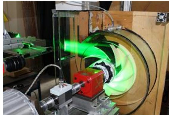
**Figure 2.** Picture of the centrifugal test rig during PIV testing.
