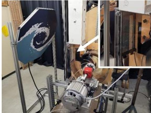
**Figure 5.** KIT centrifugal test rig and BME phased microphone array as used during the investigation.
