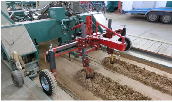
(a) The measurement setup and the sweep tool. The measurement data from the red tool on the left is used in this study.
