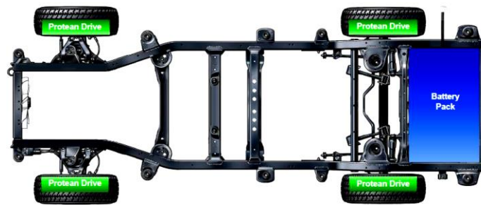
Figure 4: Chassis and drivetrain layout of a retrofitted electric vehicle with IWM (Vallance, 2011).
