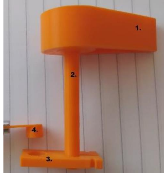
Figure 3. 3D printed pinball lever prototype (1. flipper arm, 2. flipper arm axis, 3. arm attached to pinball arm axis, 4. the link connecting the cylinder axis and the flipper arm)
