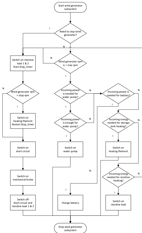
Figure 3. Wind generator subsystem flowchart
