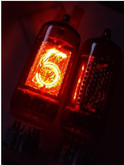
Figure 2: Fog discharge in Nixie tube
