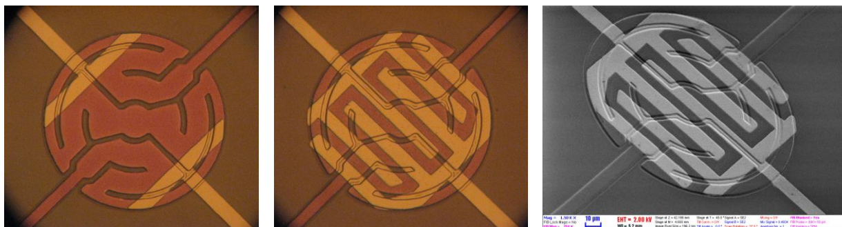
Figure 5.1. Microheaters with different electrodes for performance testing the sensitive materials.
