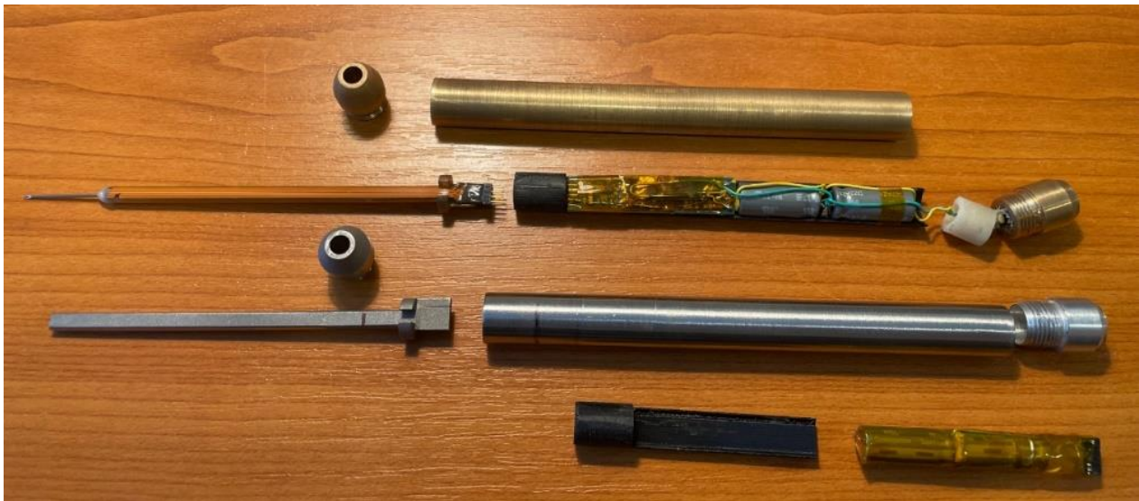
Figure 4.13. “Smart scalpel” surgical force measurement tool: head and electronics with covering
