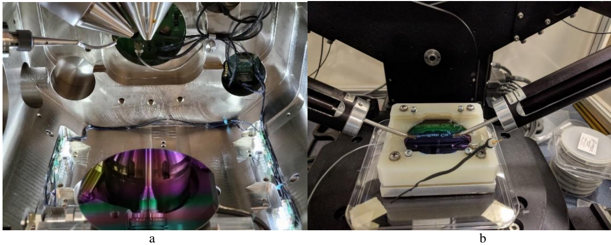
Figure 2.16. a) Combinatorial \text{TiO}_2\text{-SnO}_2 layer on a 4-inch Si-wafer in the SEM-chamber b) Electrochemical fluid cell for in-situ, real-time SE measurements.
