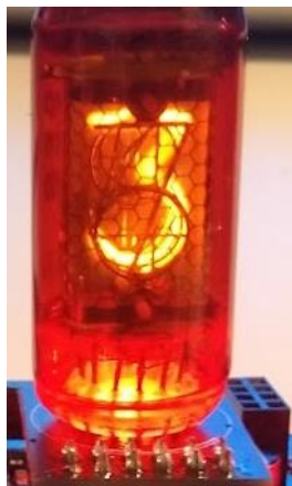
Figure 2: Fog discharge in Nixie tube
