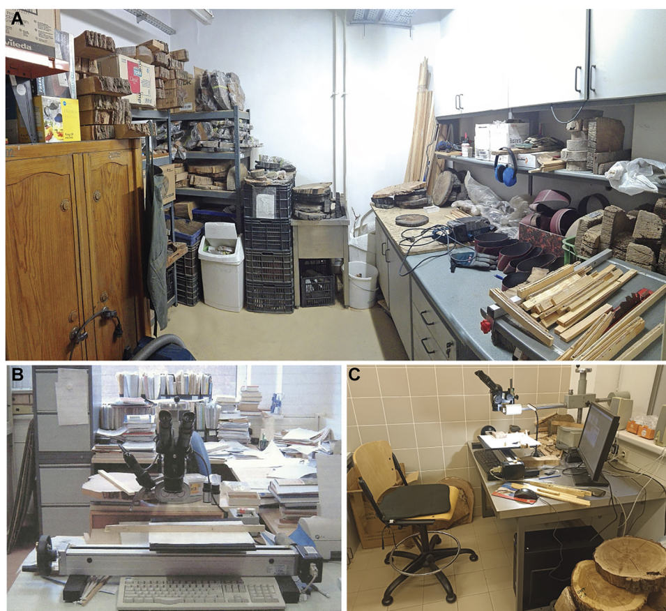
Fig. 2. Workshop for wood sample preparation and tree ring measurement stations of the Budapest Tree-Ring Laboratory. A: The workbench with the pegboard table, the sanding papers, and the sanding machine on the right side, while processed and wrapped unprocessed samples are stored on the left side of the workshop. B: The linear measuring table (LINTAB™5) with the binocular microscope as installed at the Department of Paleontology (Eötvös University) and used between 2003 and 2019. C: The tree-ring analysis instruments installed at the Department of Physical Geography (Eötvös University) and used since 2020
