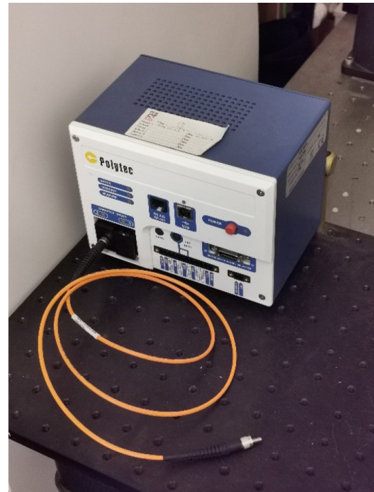
Figure 2 The Polytec CCS Prima commercial confocal sensor, equipped with an optical fiber for external supply of illumination Source: Own work
