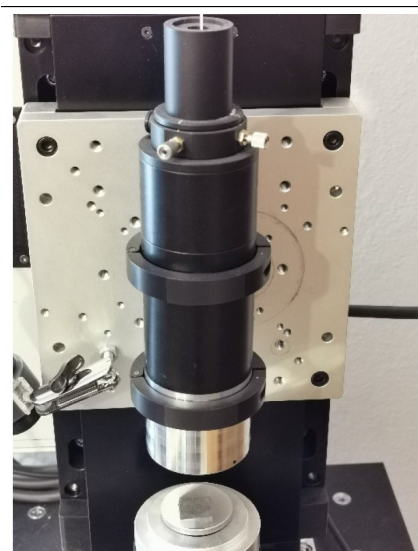
Figure 15 | The manufactured optical head, attached to the vertical actuator stage. Below the confocal probe the test mirror on the sample holder can be seen
