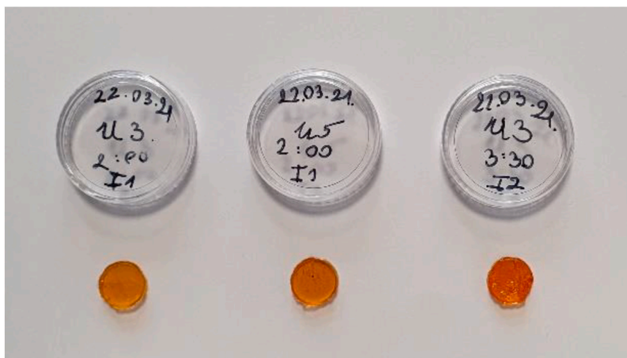
Fig. 1. Photo of some of the polymer samples prepared (from left to right: U3I1 2:00, U5I1 2:00 and U3I2 3:30). Please note the slightly deeper color of the I2 sample compared to I1 samples, caused by the higher photoinitiator concentration in the composition. (For interpretation of the references to color in this figure legend, the reader is referred to the Web version of this article.)
