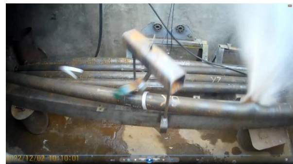
Fig. 9. The Y9 pipeline section at the end of the burst test.
