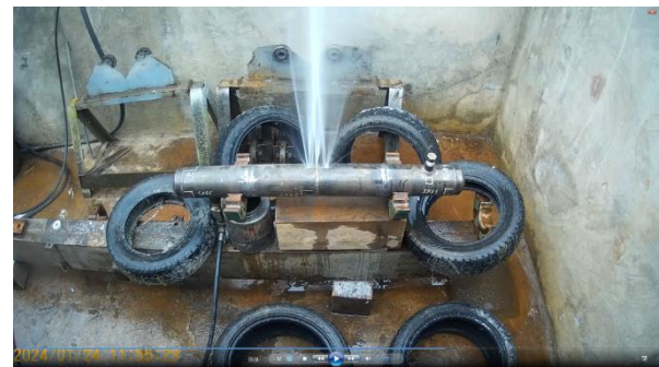
Fig. 12. The HY2 pipeline section at the end of the burst test (HY2-3).
