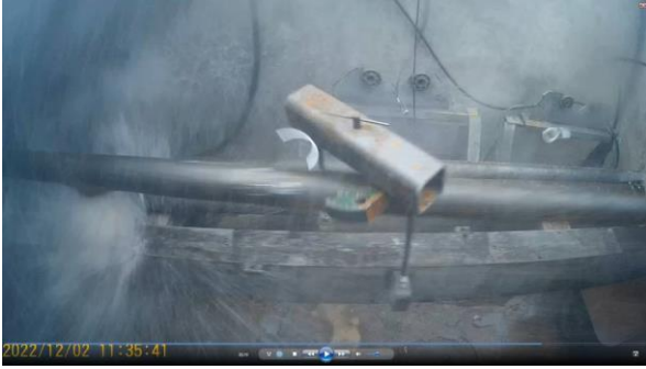
Fig. 10. The Y10 pipeline section at the end of the burst test.
