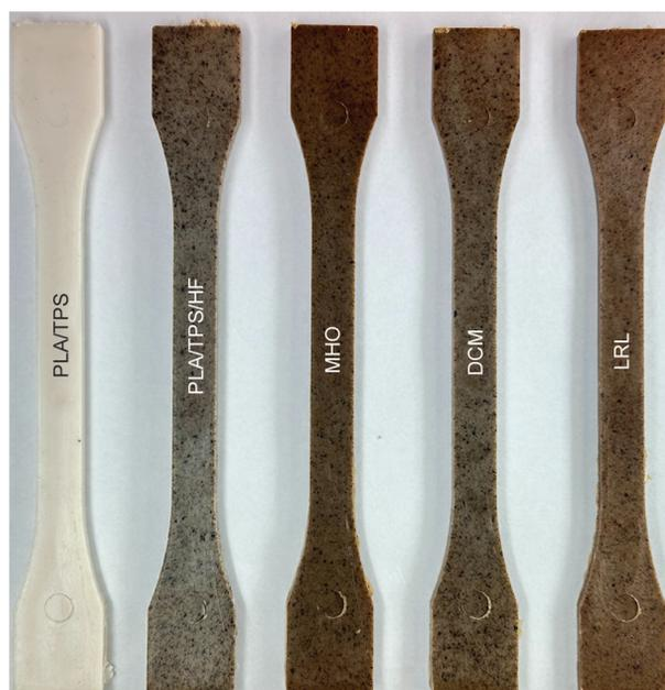
**Figure 10.** The visual appearance of PLA/TPS samples and PLA/TPS/HF samples without compatibilizer and compatibilized PLA/TPS/HF samples.
