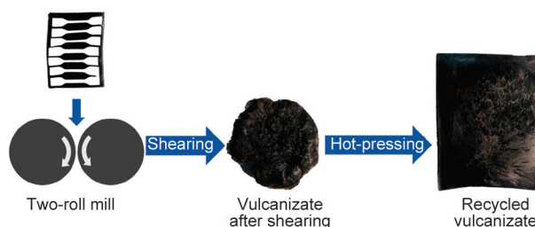
Figure 12. Schematic diagram of recycling method of vulcanizates.
