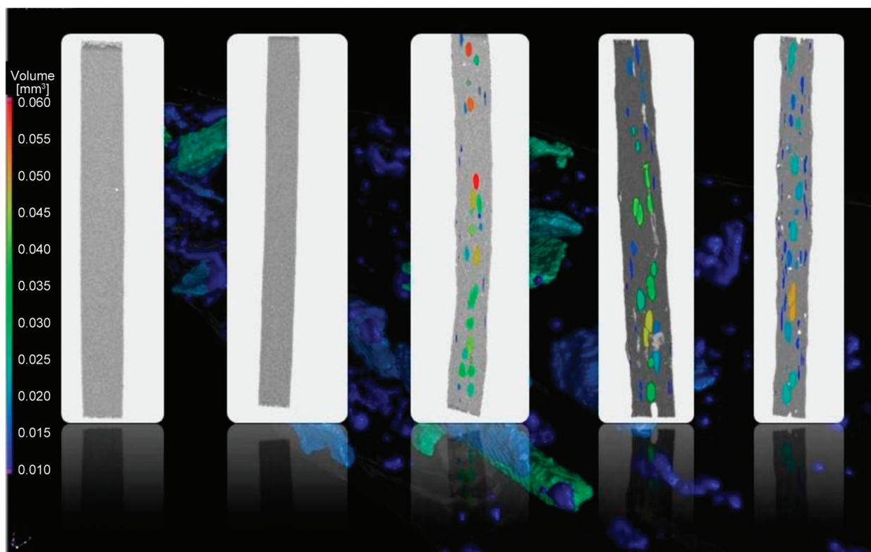
**Figure 8.** 2D slices produced from the 3D CT measurement of extruded samples. Coloured surfaces characterize the micro-porosity of the samples, while bright surfaces (white colour areas) belong to the inclusions. The image used as background is the 3D visualisation example of inclusions in the SR sample. (2D images characterize the results of B, BCL, SI, SR and RDF samples from left to right).
