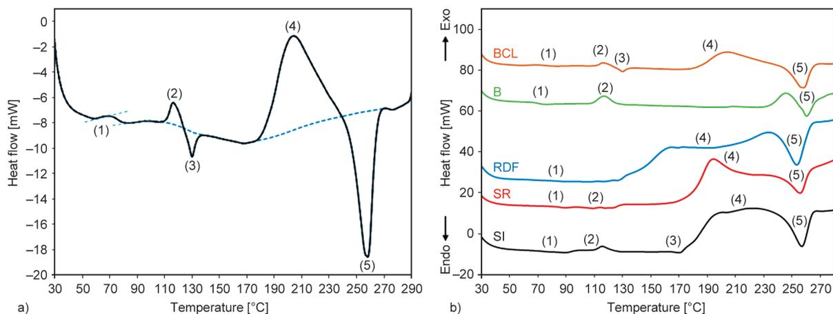
**Figure 4.** The DSC analysis and evaluation (BCL (a)) of the shredded PET waste samples (b). (1):  $T_g$  – glass transition; (2):  $T_{cc}$  – cold crystallization; (3):  $T_{endo}$  – endotherm peak, polyolefin component melting; (4)  $T_{exo}$  – exothermic peak, polyolefin component phase transition and (5):  $T_m$  – melting. (SI – selective income; SR – sorting residue; RDF – refuse derived fuel; B – bottle; BCL – bottle with cap and label).
