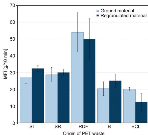
**Figure 5.** MFI values of PET wastes from different sources and with different pretreatment. (SI – selective income; SR – sorting residue; RDF – refuse derived fuel; B – bottle; BCL – bottle with cap and label).
