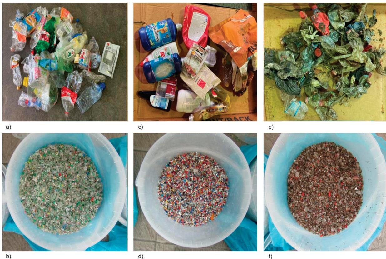
**Figure 2.** NIR separated and shredded PET samples from real waste a) SI, b) shredded SI, c) SR, d) shredded SR, e) RDF, f) shredded RDF (SI – selective income; SR – sorting residue; RDF – refuse derived fuel).
