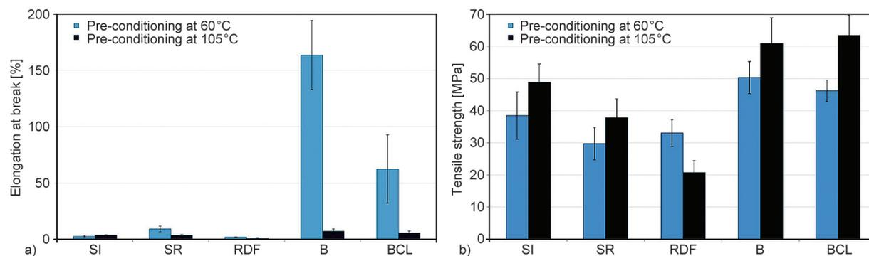
**Figure 7.** Elongation at break (a) and tensile strength (b) of extruded PET wastes from different sources. (SI – selective income; SR – sorting residue; RDF – refuse derived fuel; B – bottle; BCL – bottle with cap and label).
