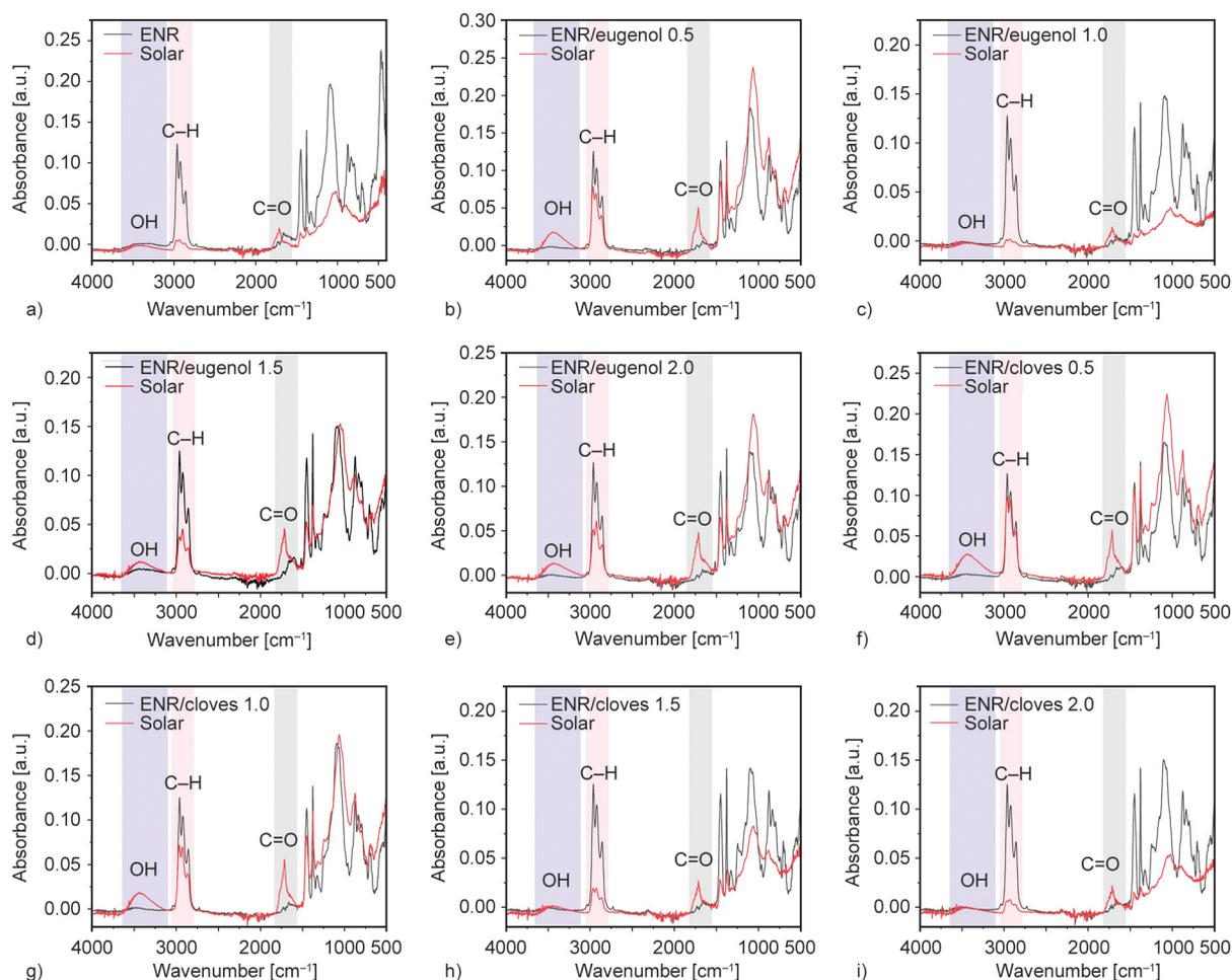
**Figure 5.** FTIR spectra of ENR (a), ENR with eugenol (b–e) and ENR with cloves (f–i) before and after solar aging.
