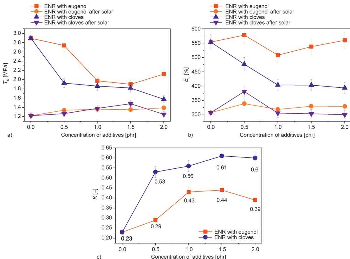
**Figure 4.** Mechanical properties: a) tensile strength ( $T_S$ ) and b) elongation at break ( $E_b$ ) before and after solar aging; c) aging coefficients  $K$  of materials.
