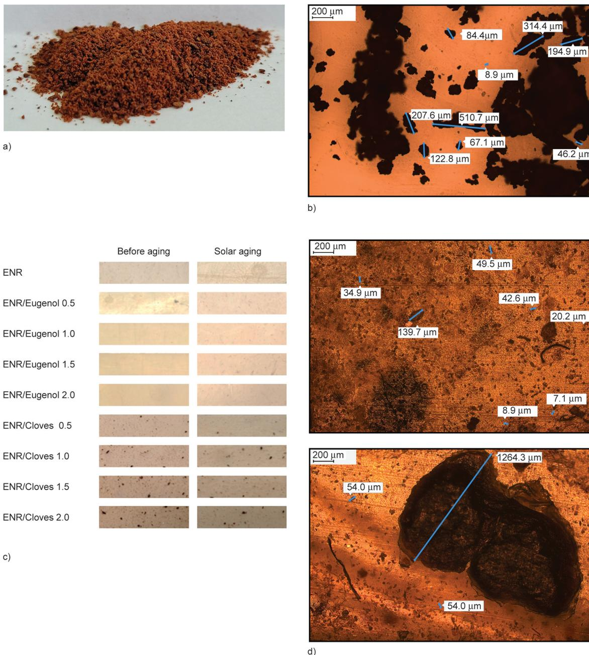
**Figure 1.** Photos of ground cloves: a) photo from a camera, b) photo from an optical microscope with 100 $\times$  magnification. Photos of ENR samples: c) photos of samples from a camera before and after solar aging, d) photos of ENR/clove samples from an optical microscope with 100 $\times$  magnification. Blue arrows mark the lengths of clove particles in the photos (5–1200  $\mu\text{m}$ ).
