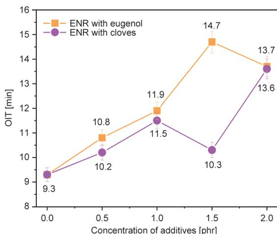
**Figure 3.** Oxidation induction time (OIT) of ENR composition with eugenol and cloves.
