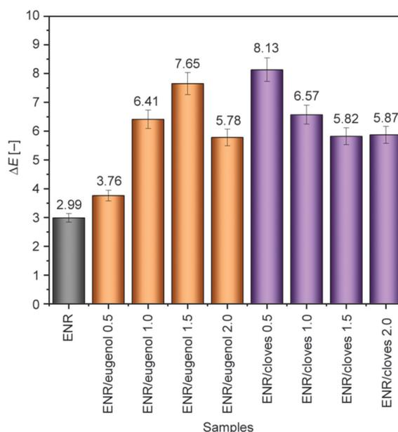
**Figure 7.** Change of color ( $\Delta E$ ) of ENR samples with eugenol and cloves during solar aging.
