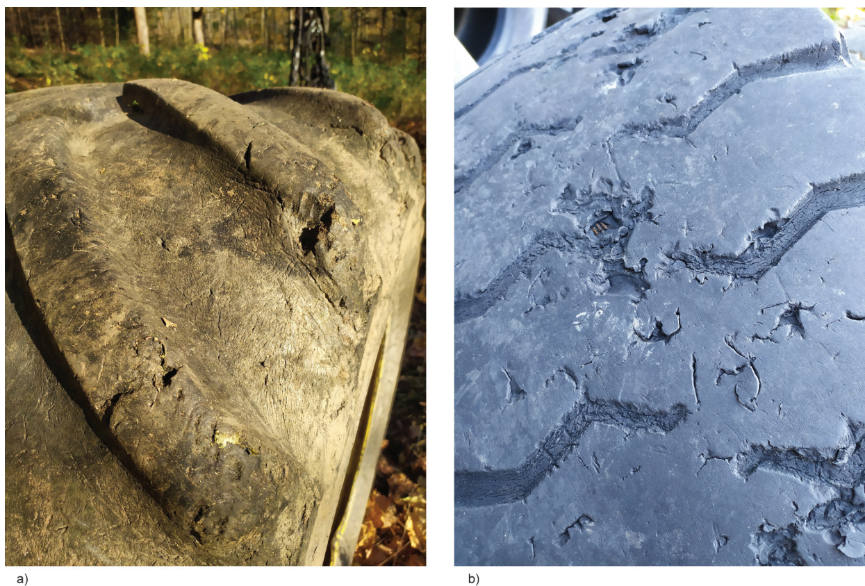
Figure 1. Photographs of the worn tire treads illustrating the CC wear mechanism: forestry equipment tire (a), and MPT (b).
