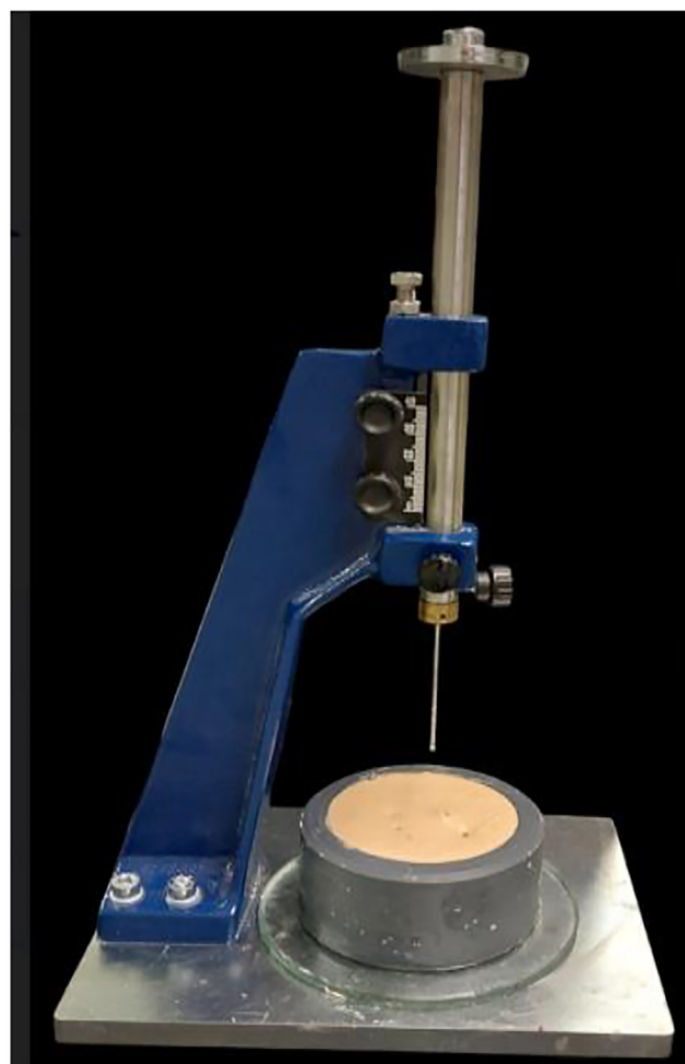
Fig. 1. Vicat apparatus for the measurement of geopolymer binder test (Source: Authors' photo)
