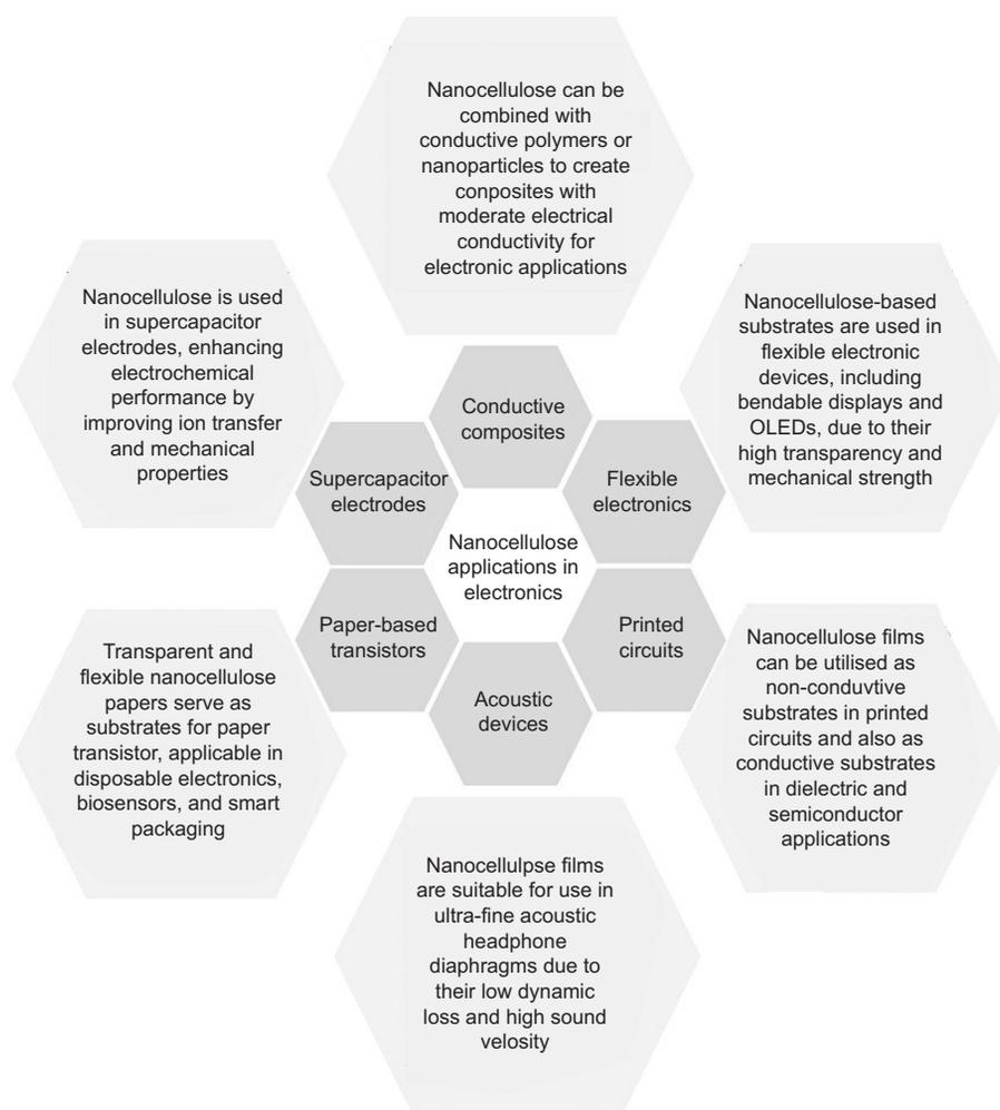
Figure 5. Nanocellulose applications in electronics.
