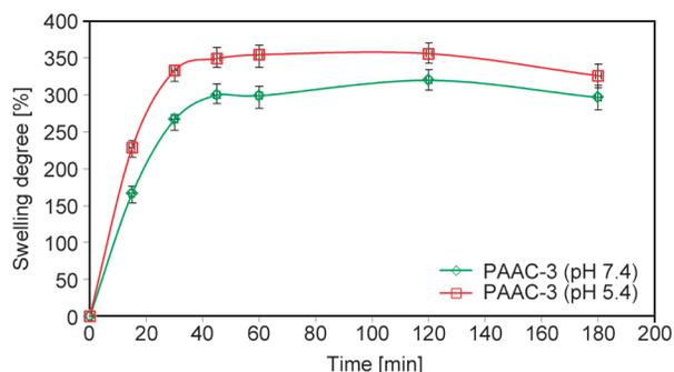
Figure 7. Swelling degree of the PAAC-3 nanofibers in solutions with pH 7.4 and pH 5.4.
