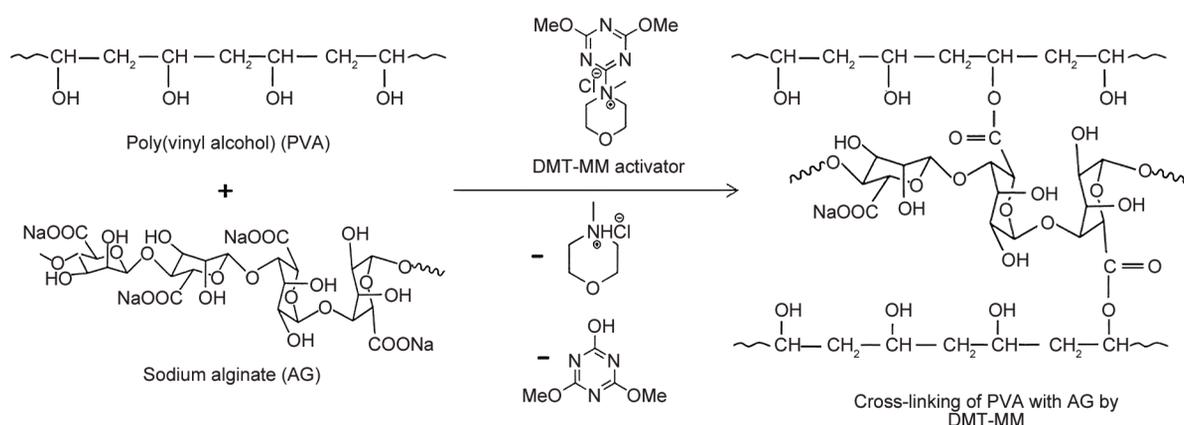
**Figure 1.** Esterification reaction of PVA with AG in the presence of DMT-MM activator.
