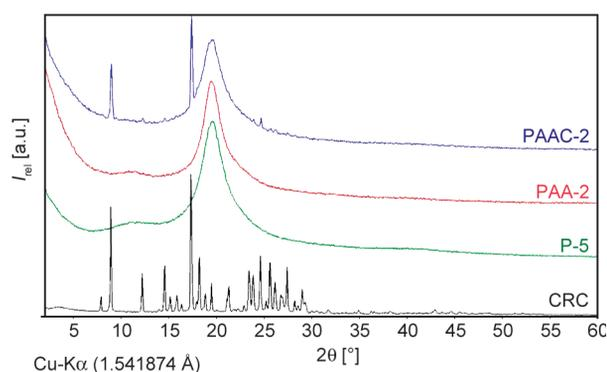
**Figure 3.** XRD spectra of pure CRC, nanofibers without CRC (P-5 and PAA-2) and nanofibers with CRC (PAAC-2).
