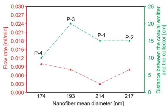
**Figure 6.** Relationship between the nanofibers' mean diameter and solution flow rate and distance between the coaxial emitter and the collector.
