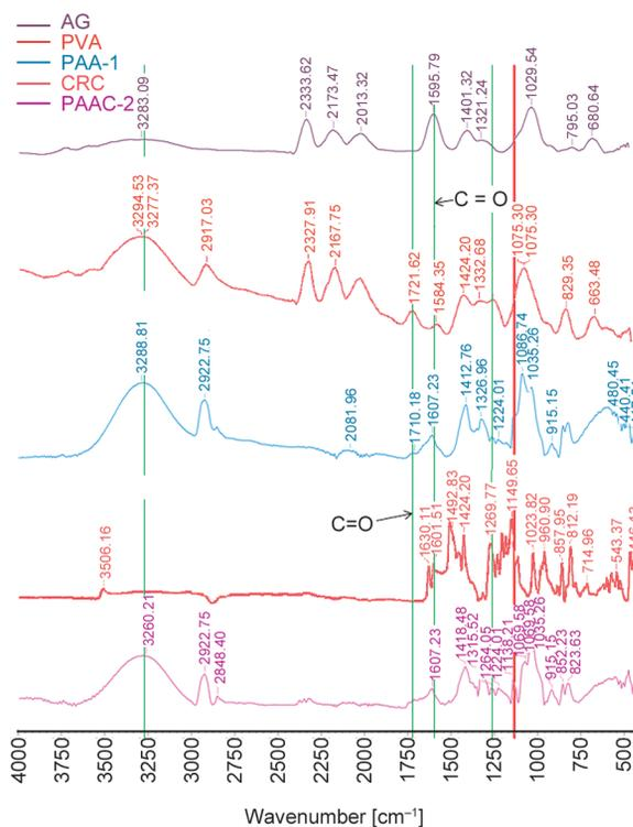
**Figure 2.** FT-IR spectra for simple CRC, nanofibers without CRC (PAA-1) and nanofibers with CRC (PAAC-2).
