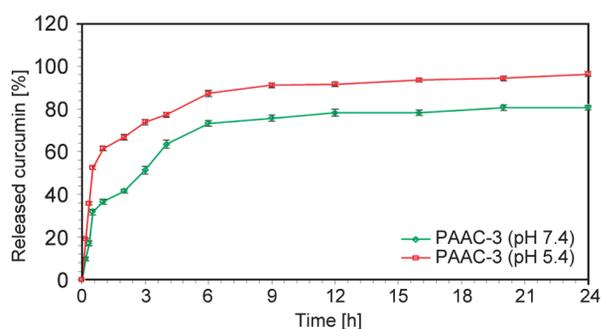
Figure 8. *In vitro* release degree of CRC from PAAC-3 nanofibers in PBS solutions (pH 7.4, pH 5.4).
