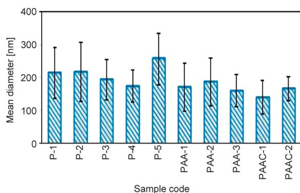
**Figure 5.** Nanofibers mean diameters depending on the molar ratio between the two polymers.
