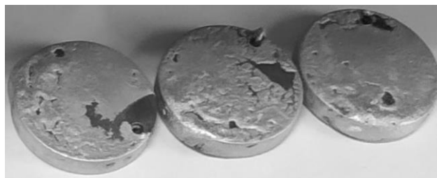
Figure 1 Photos of three aluminized steel samples produced by the laboratory hot-dip aluminizing at 2.5 min. dipping time
