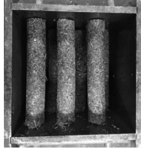
Figure 3 The reed seeds in the mould
