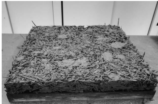
Figure 6 Thermal insulation reed panel
