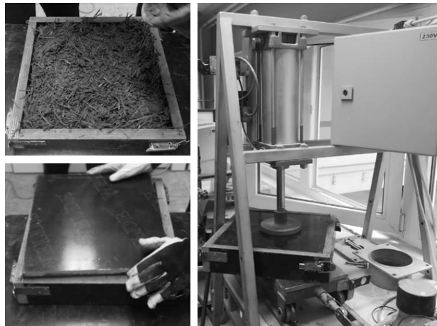
Figure 4 The process of pressing a reed panel
