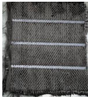
Figure 1: PCL interlayer material 3D printed directly on the reinforcement material.
