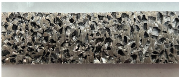
Figure 3. Aluminium foam made by the granular method.
