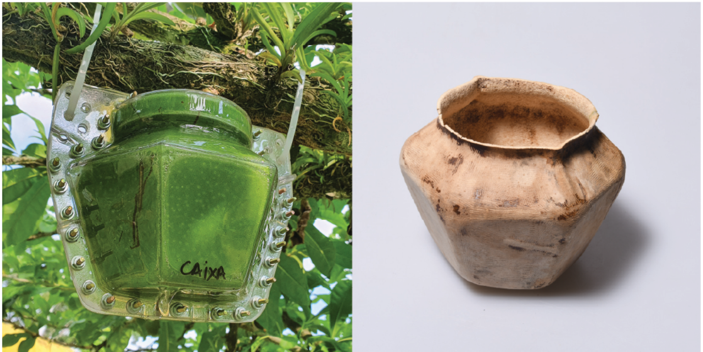
Figure 4. Cuia Colab prototype being molded (left) and the harvested object (right). Source: Andrea Bandoni, 2022.
