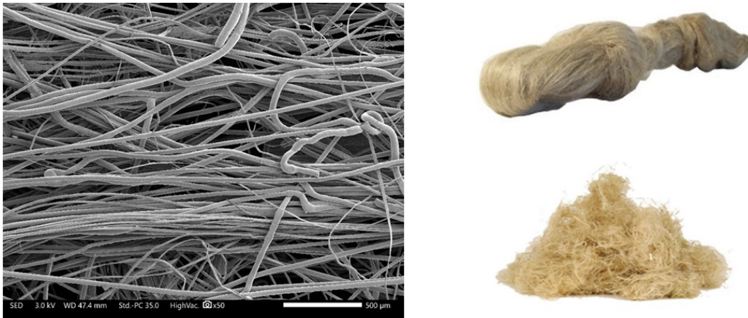
Figure 5. Images from the project Flower : Long natural flax fibers are broken into shorter ones to be integrated as matrix inside a composite material.
