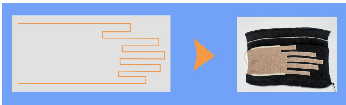
Figure 5. Flat pattern design with conductive path and knitted flat pattern. In this pattern, we used a 90° rotation of the glove.
