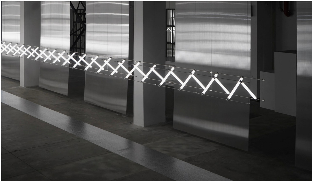
Figure 1. Mario Tsai' Mazha system. The conductive transmission of low voltage across the structure of the lighting allows the lamp to be free from wires and to build diverse and endlessly changing systems with free units. Based on these theoretical and technical foundations, the first generation of modular lighting systems in the Mario Tsai studio was inspired by the traditional Chinese sitter Mazha Lighting System.
