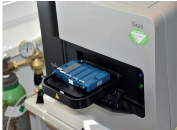
Figure 3. Illumina iScan instrument for the reading of beadchips
