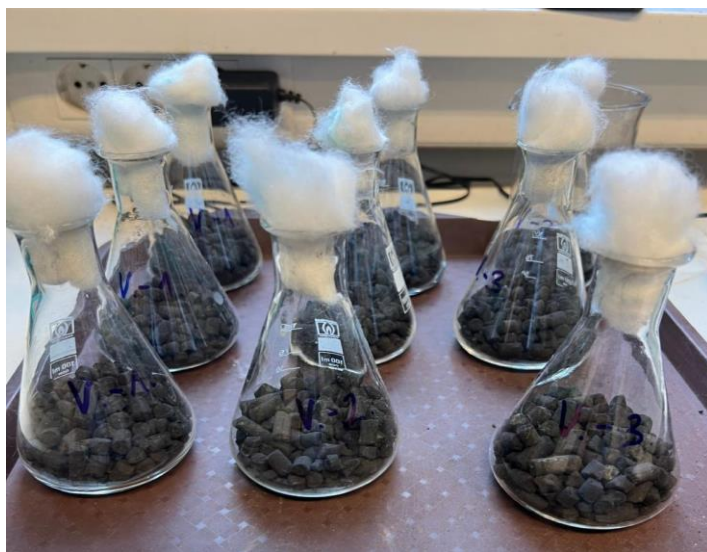
Figure 1. Sterile Erlenmeyer flasks containing 40 g of each biochar sample were used before microbial inoculation
