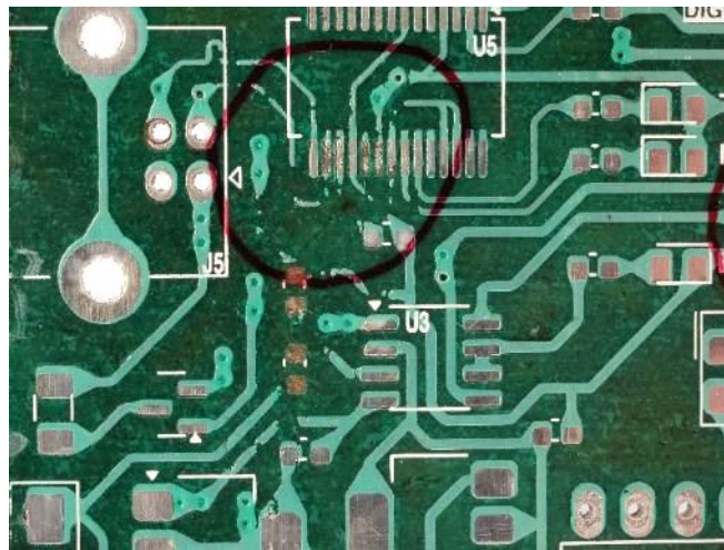
Fig 6. Opens in the wiring due to insufficient masking
