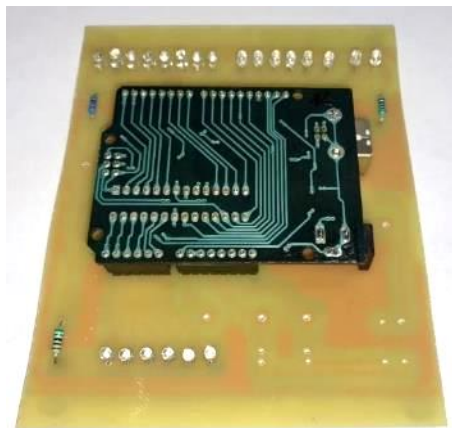
Fig. 18. Simple test circuit for the Biodegradable Uno
