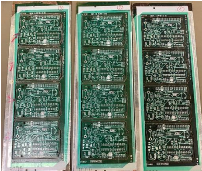
Fig 15. Panelized PCB frames based on the new design
