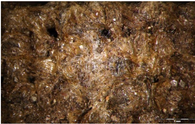
Fig. 12. White filaments found with optical microscopy on bare dielectric samples. 43th week.
