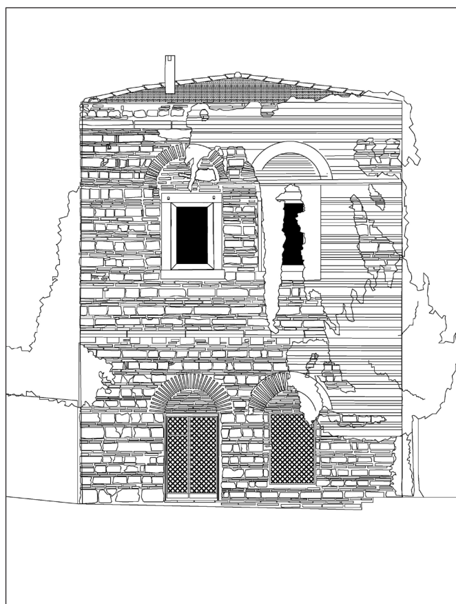
Fig. 6. Digital survey drawing of the south-eastern façade of the Transylvanian Ambassadors' House (Made by: Róbert Kulcsár-Kilyén, 2019)
