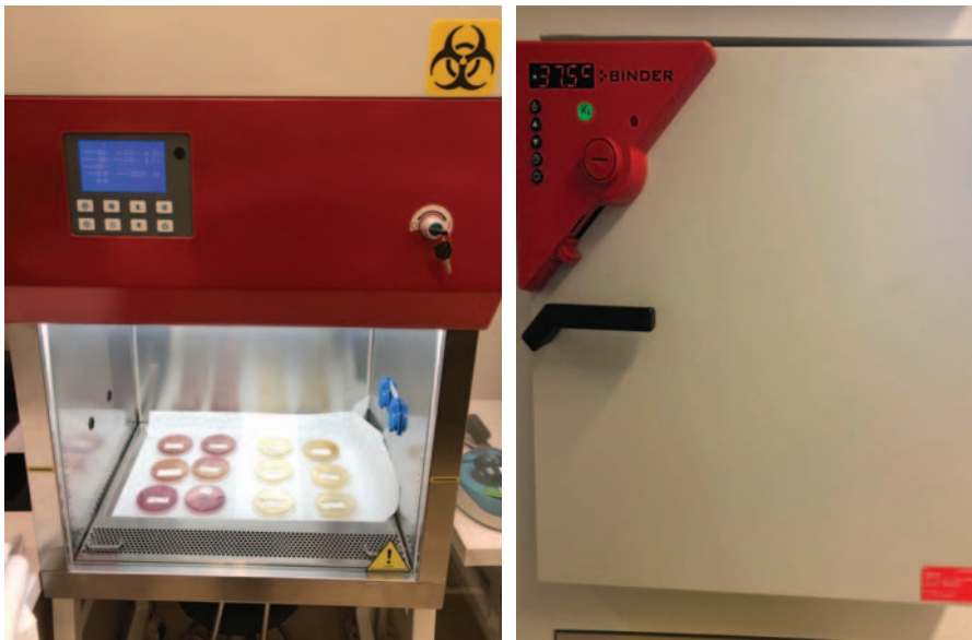
Figure 6. On the left, aspect of the Fagronlab Class II Biological Safety Cabinet equipped with two HEPA filters, from the Laboratory of the 2 nd Author (Dr Elsa FAVIOU, MD). The HEPA filtered downward laminar flow protects the material used inside the cabinet and the exhaust HEPA filter protects the Environment since it ensures that the air passing through is contaminants' free. The working area is surrounded by negative pressure. Mac Conkey Agar and SGC2 Agar (Biomérieux S.A.) were used for the culture of bacterial and fungal inocula. On the right, aspect of the Lab-Incubator (Binder), used for culture growth. Because of its precise temperature accuracy (0.1 °C; it also fulfills the temperature safety requirements according to DIN12880) this device is especially useful for incubation of cultures at a standard temperature of 37 °C (98.6 °F). © Copyright by the authors. Courtesy of Dr Elsa FAVIOU, MD.
