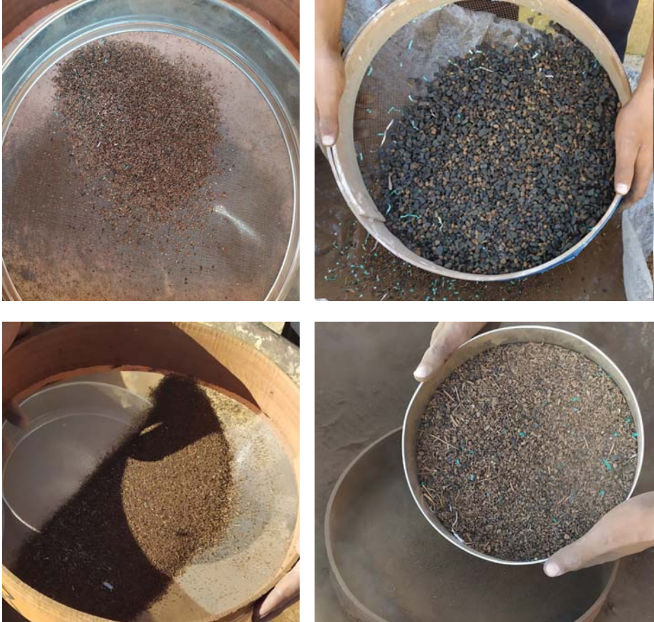
Figure 8. Sieving samples after flotation and different sizes of samples
