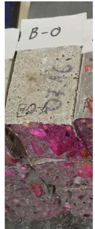
Figure 5: CEM II specimens after the acid test
