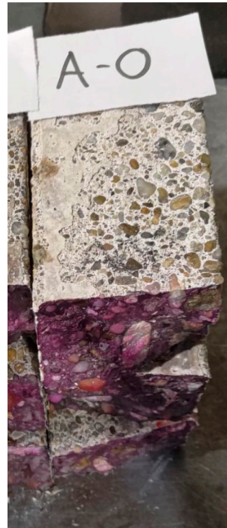
Figure 4: CEM I specimens after the acid test
