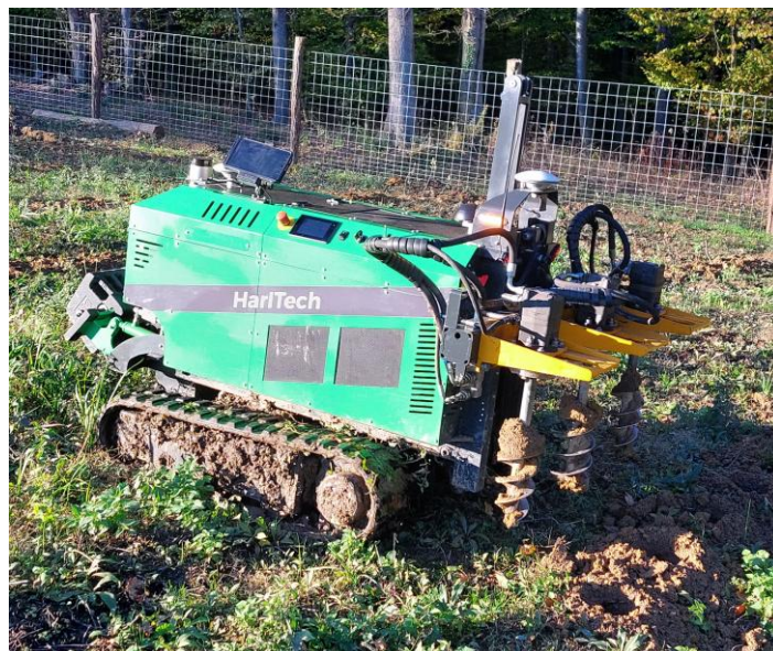
Figure 1: The haRiBOT V3 self-propelled robot at work
