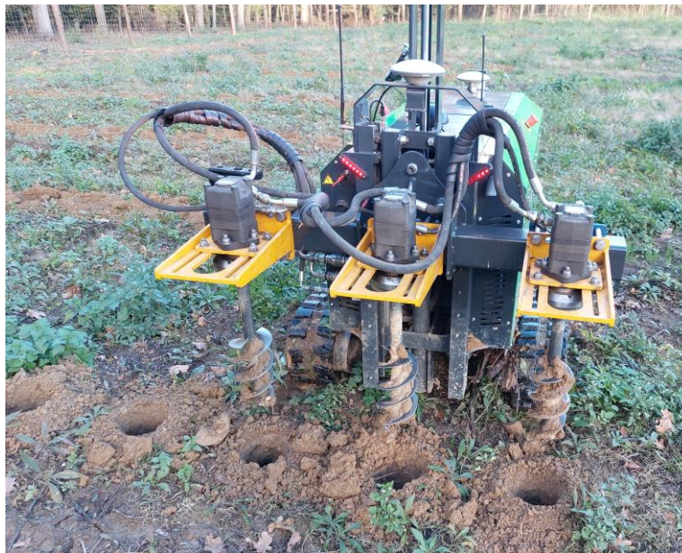
Figure 5: Application of three auger heads operating perpendicular to the rows
