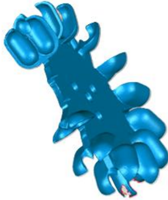
Figure 5. Scanned 3D geometry of impeller
