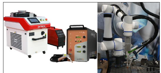
Fig. 3. Hand-held laser sources (left) and their integrated system with a robot (right) [6]
