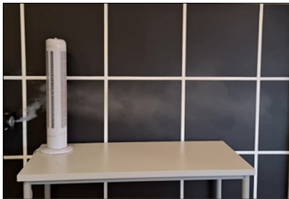
Fig. 13. Smoke test of the tower fan.
