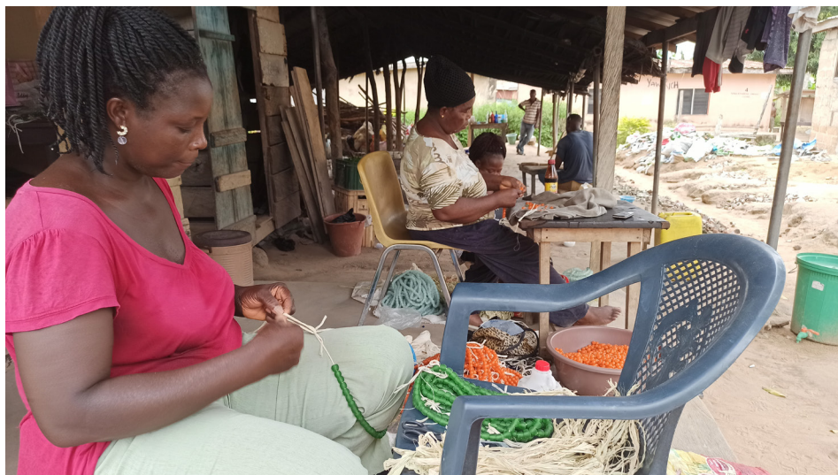
14. Women can have different roles in the beadmaking process, such as filling molds with powdered or crushed glass, creating motifs by pouring glass powder of different colours into the mold or by painting, and stringing beads for sale.
