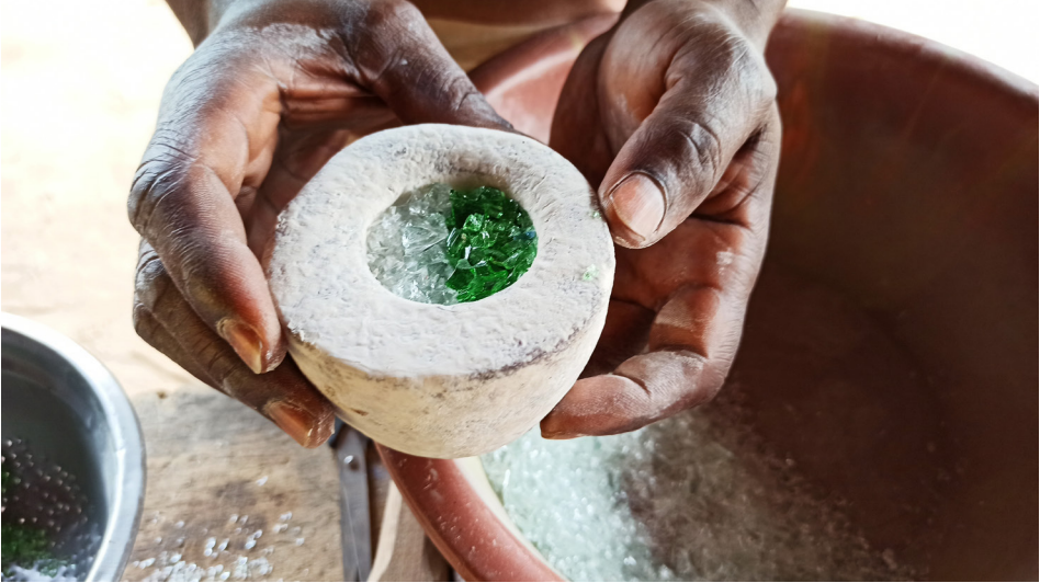
11. By placing crushed glass of different colours in the mold, multicoloured translucent beads can be created
