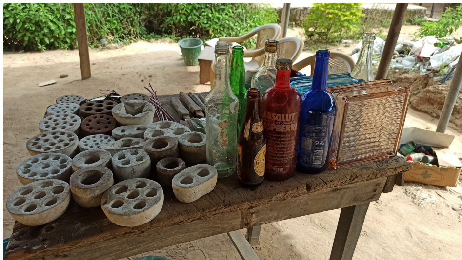
9. Set of raw materials and tools for making translucent beads from fragments of broken glass, retaining the original colours of bottles or industrial glass products
