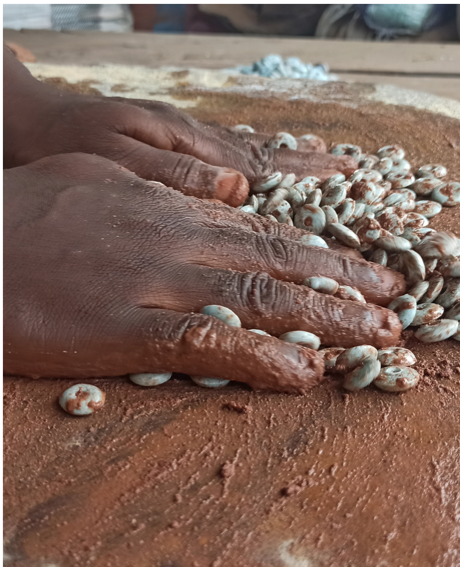
8. Polishing beads with fine sand and water on a grinding stone
