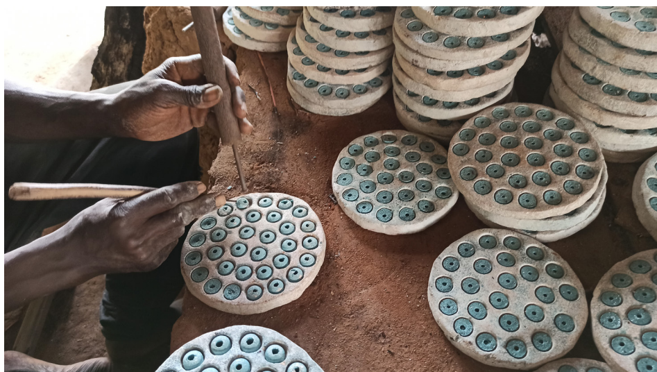
6. Turning each bead after the first firing and placing it in the kiln for a second, shorter firing to achieve a domed surface on each side
