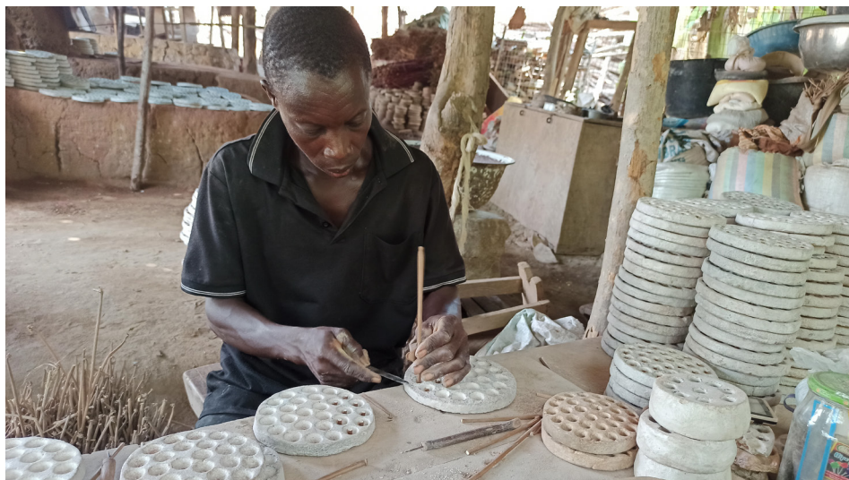
4. Inserting cassava leaf stalks into the holes of the mould to form the bead holes after firing
