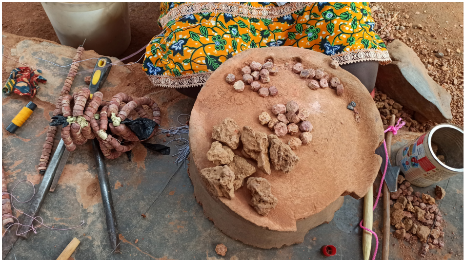
16. Abompeh is the only settlement in Ghana where bauxite beads are made, thanks to a nearby bauxite mine. Simple tools are used, and holes are drilled with a bow drill. Because of their red colour, bauxite beads are mainly worn at funerals and during mourning. Abompeh, 14 April 2023
