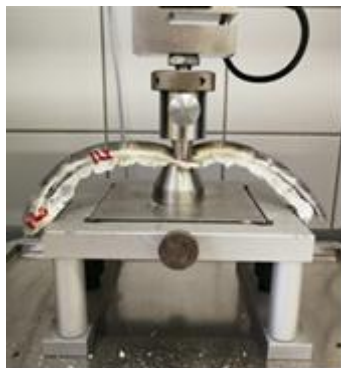
Figure 4 Hoof sample during measurement
