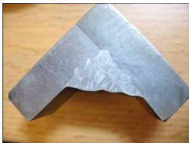
Figure 3. Welded joint, polished and etched.
