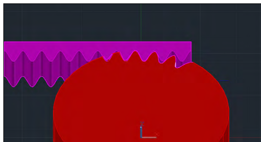
Figure 10. The subtracting operation through the rolling process.
