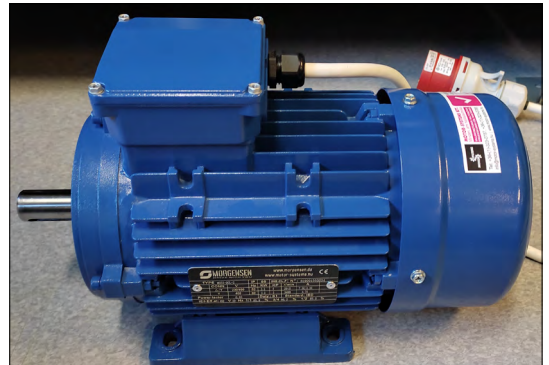
Figure 5. Electric motor for driving the generator.
