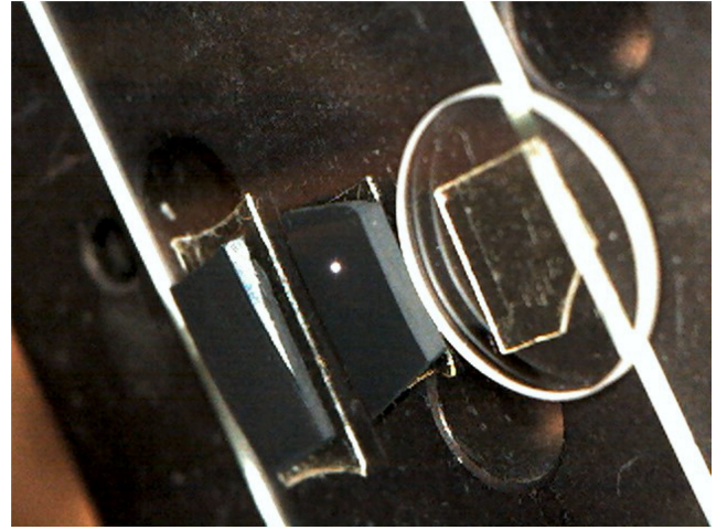
Figure 20: Test samples used to evaluate the performance of the prototype system on real-life specimens, imaged with a microscope camera attached to the measurement setup. From left to right: a microstructured surface of an elastomer seal, the flat surface of the same elastomer seal, and an antireflection-coated optical window. The focused infrared beam of the microscope is visible on the surface of the central (flat elastomer) sample.
