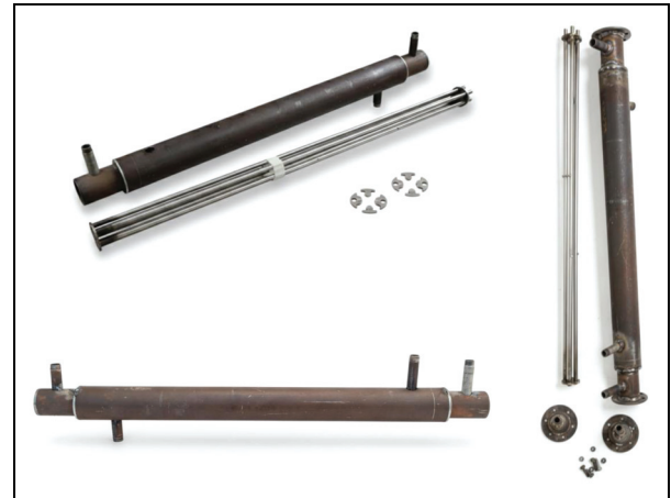
Figure 10. Fabricated prototype of the double-shell heat exchanger with internal components.
